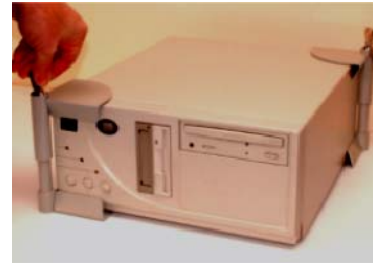
Cornerlox traps the PC by two diagonal corners
