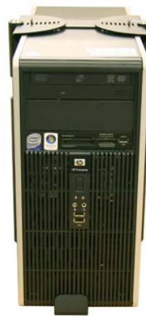
Adjustable tie bars for towers prevents the clamps being forced apart
